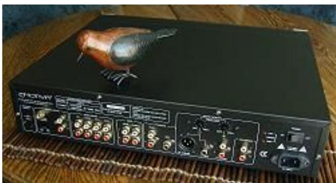
You can see on the rear panel photo above that the full-range output jacks are situated next to the split-output jacks, and that the low-pass (for the subwoofer) offers both an RCA unbalanced as well as an XLR balanced output. The low-pass output combines both channels and comes from an op-amp, while the high-pass output is the main preamplifier output stage with a filter.
