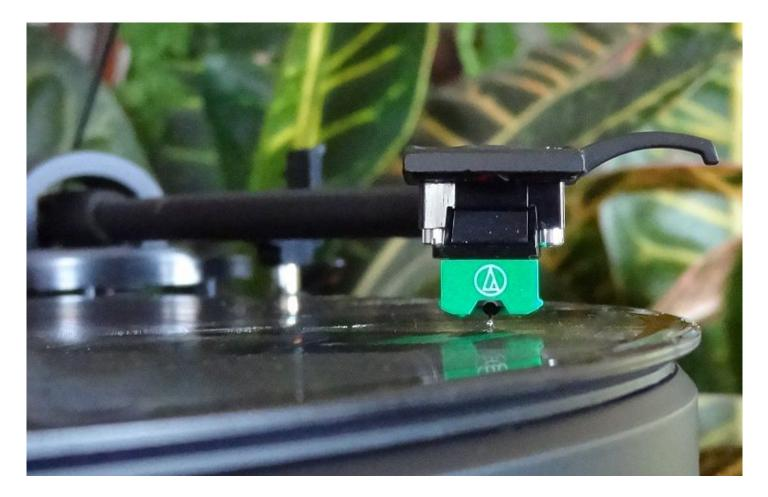
Fourth, the Horizontal Tracking Angle, also known as the Zenith, is set by adjusting the mounting screws that hold the cartridge in the headshell so that the cartridge is perpendicular to a line drawn from the center hole of the LP to the outside edge, and a line drawn through the body of the cartridge (front-to-rear) as the stylus is in the groove.
