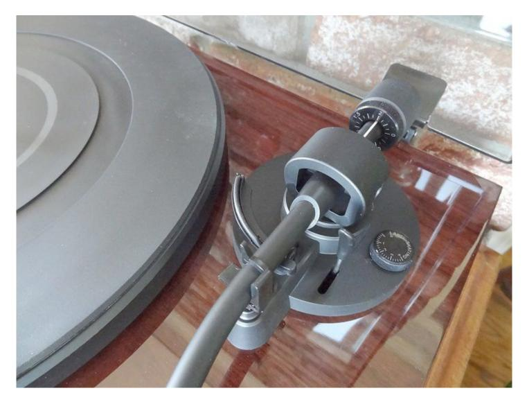
Secondly, the Vertical Tracking Angle (VTA) is the tilt of the tonearm as the cartridge stylus is in the groove of an LP.
