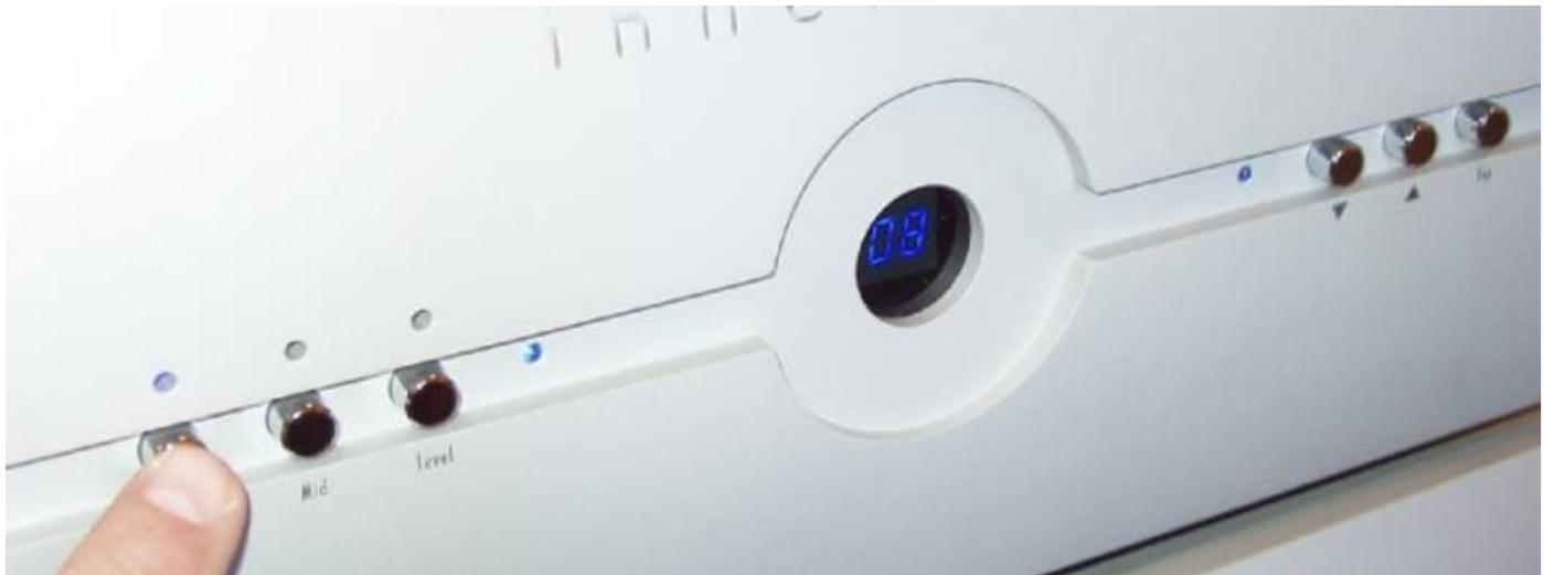
Using the up and down arrows on the right, you adjust the amount of bass. This just changes the bass, not the mid-bass (which is adjusted by use of the Mid button). The overall volume is adjusted by the Level button.
