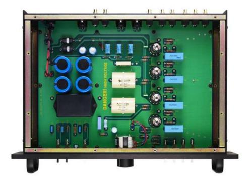
The photo below shows a close-up of the four 6H30 tubes in the control chassis. They have silicone rings around them to limit microphonics (vibrations that cause electrical noise). Notice also that the tube sockets are mounted on small posts rather than being flat against the circuit board (see inset for detail).
