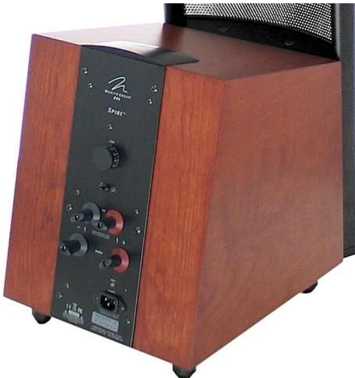
Here is a close-up of the dial, and you can also see the jumper clips that connect the ESL panel to the woofer. There is a small toggle to turn off a blue MartinLogan logo that is on the top of the woofer enclosure, as it can be seen through the translucent ESL panel.
