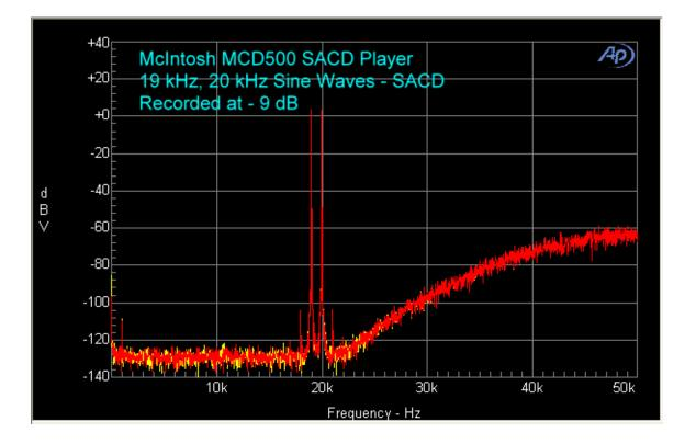
The IMD measurements were 0.005% for CD, and 0.08% for SACD.
