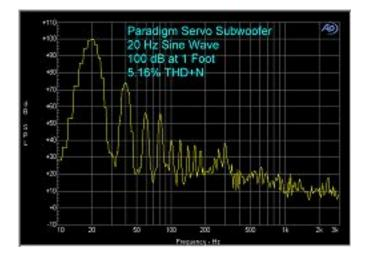
THD+N vs. Frequency indicated that distortion stayed at 5% or below from 15 Hz to 200 Hz.
