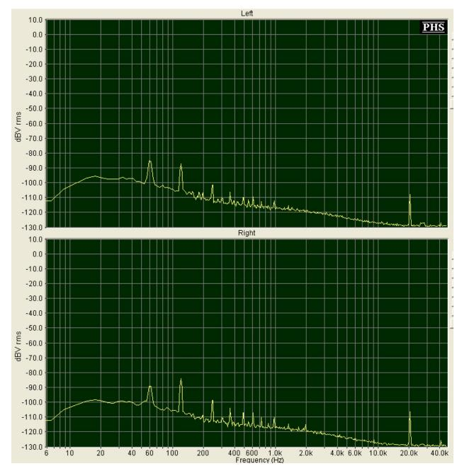
With the 65 dB gain setting that I used with the Sumiko Starling low output (0.5 mV) moving coil cartridge, the noise level is much higher. This is the compromise that has to be made with a low output cartridge. What you get in return is more detail, because the cantilever is lighter (the number of turns on the coils is lower, which results in lower
