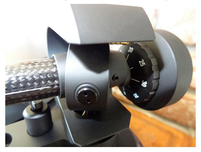
When the screw is loose, you rotate the tonearm until the cartridge cantilever is vertical when resting on an LP. Note: raise the tonearm with one hand and rotate it with the other hand. *Do not* rotate the tonearm while the stylus is resting on the LP. Once it is vertical, tighten the hex screw (with the tonearm raised).
