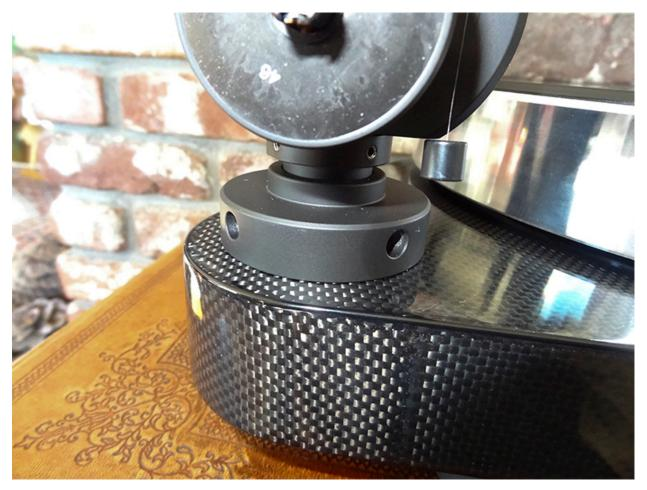
To do this, you insert the hex wrench in the two sockets, loosen the hex screws (hold on to the tonearm so that it does not collapse down onto the LP), and then move the tonearm up or down until it is level (the space between the tonearm and an LP), as shown in the photo below.
