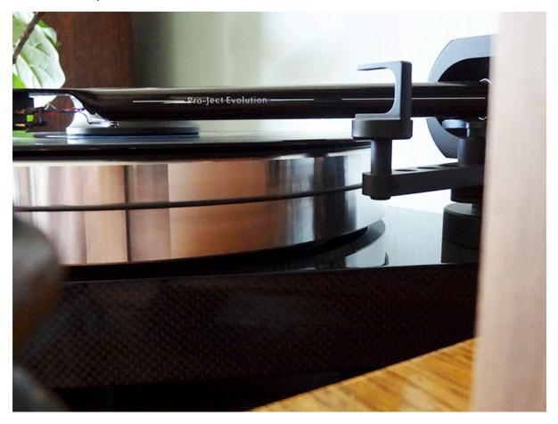
The **Azimuth** refers to having the cartridge not tilted to the left or right, i.e., when looking at the front of the cartridge, not having the left side closer or farther from the surface of the LP than the right side, and more specifically, the cantilever is vertical.
