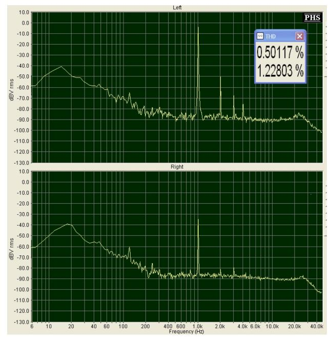
I tested the cross-talk (channel separation) by using a 1 kHz sine wave only in the left channel. There was no groove signal in the right channel.
