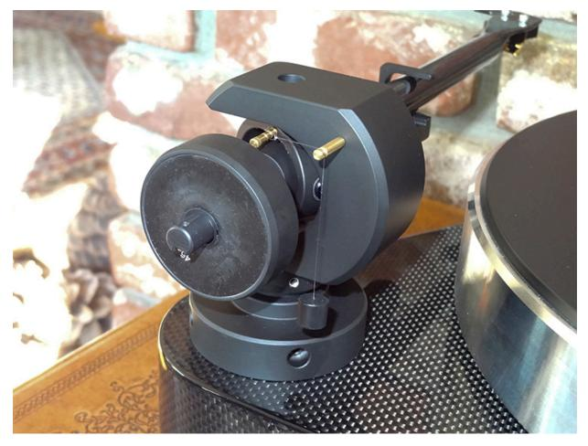
You can see the rod at the top, center, which is attached to the tonearm. The Anti-Skate filament is looped over that rod and also the rod on the right, center, then the weight is suspended.
