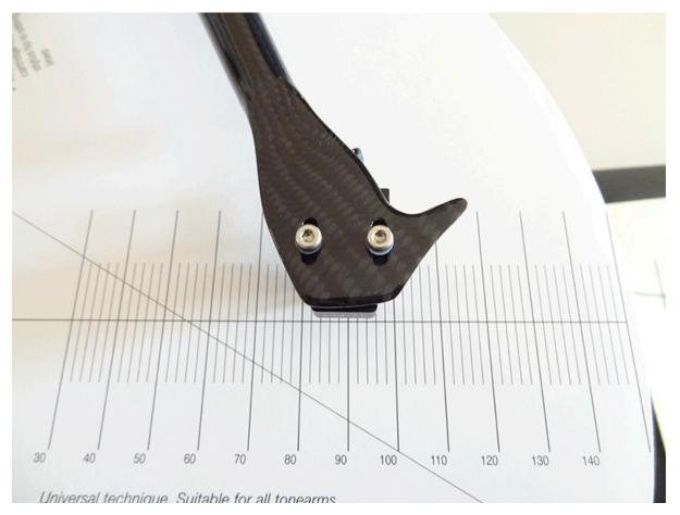
The cartridge moves in an arc across the LP, so it is only at the proper tangent at one place. You have to choose where that place is. I chose a spot that is midway between the outer edge of the LP and the beginning of the lead-out groove at the end of the LP.
