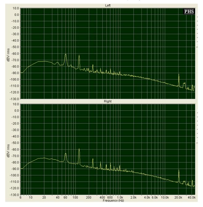
I used the subsonic filter because it reduces the low frequency noise below 20 Hz.
