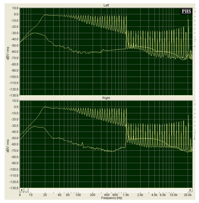
You can see the response is flat up to about 12 kHz and then begins to rise. This is not uncommon. The dip at 18 kHz is probably an artifact. The response drops rapidly below 20 Hz due to the subsonic filter that attenuates beginning at 20 Hz and increases at 12 dB/octave below 20 Hz.
