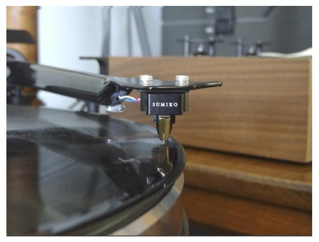
When playing an LP, there is a tendency for the stylus to move towards the center spindle because the grooves near the center are rotating at a lower linear velocity than grooves near the outer edge (the inner grooves are smaller diameter).
