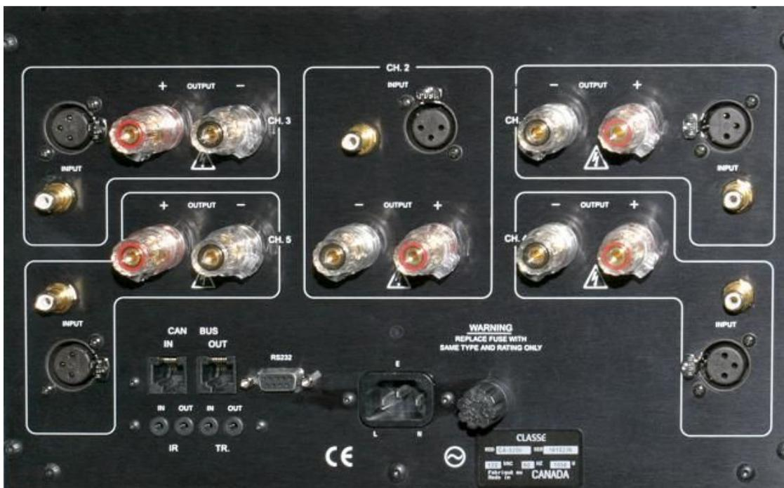
The back panel also has jacks for triggering on/off, a bus to connect several amplifiers together so that they can all be turned on in sequence, and an RS232 port for upgrading software down the road.
