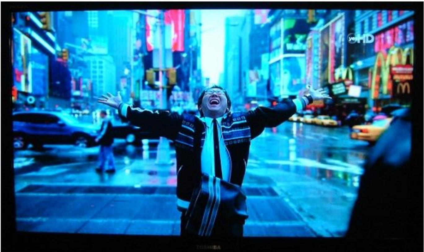
Low light scenes in *The Fifth Element* required me to turn the black stretch feature back on. Not doing so caused both banding and reddish grain and turning Lilo's face into a dithered red mess. It was quite a bit better with black stretch on, but still not nearly as nice as some of the other displays I have tested using that very same scene. The black guard uniforms were virtually undetailed, as all the black detail was simply clipped by the contrast enhancement that this display offered.
