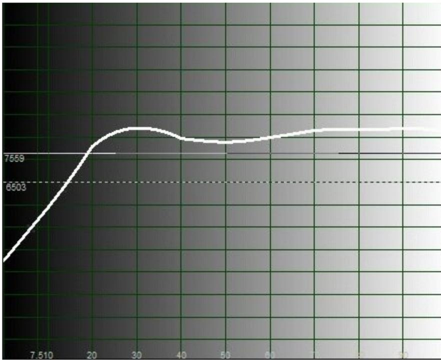
The RGB levels. Remember that I said it looked too blue? Here is the proof. Note that this does not conflict with the CIE chart shown below where it indicates that the blue is undersaturated with respect to the HDTV standard. The blue can be turned up too high without being “saturated” enough.
