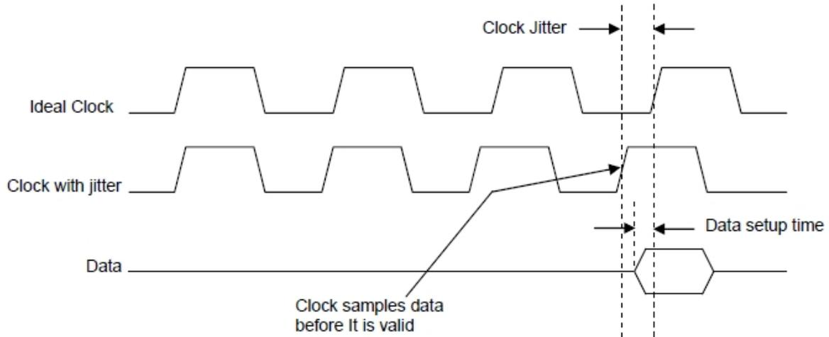
The data hold time is the amount of time that a bit needs to be held in order to be read. If the bit comes too late, again, the microprocessor receives incorrect information.
