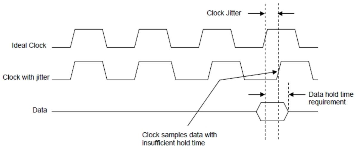
This is not a paper on jitter, so I won't go into the other types. Just be aware that jitter is an important issue to be addressed in digital audio. That is the function of the clock that comes standard with the Auralic VEGA G2 and is superbly addressed with the Auralic
