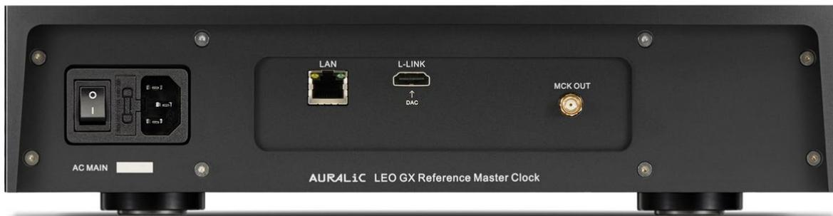
The Master Clock In (MCK IN) on the VEGA G2 is connected to the MCK OUT on the LEO GX. This is the main communication from the LEO GX to the VEGA G2. There is also a Lightning Link (L-Link) connection between the two components. I connected them using the included cable (HDMI). This provides jitter-free communication between Auralic components.
