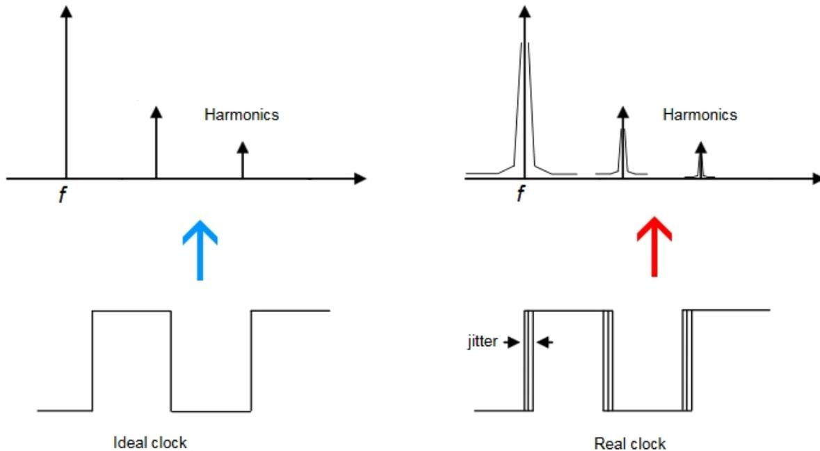
With a perfect (Ideal) clock, the 1's and 0's have no jitter, i.e., the timing is as it should be, shown in the left-hand side of the diagram. Frequencies in the music, and their harmonics, are narrow peaks. With the real world (Real Clock), the 1's and 0's do not arrive exactly when they should, and the frequencies in the music, and their harmonics, appear with widened peaks, especially at the base (right-hand side of the diagram). Some of this is side-band peaks, distorting the music.
